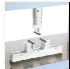
3-point bending test of plastic specimen
